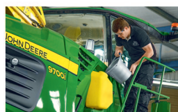
Additive dosing system
